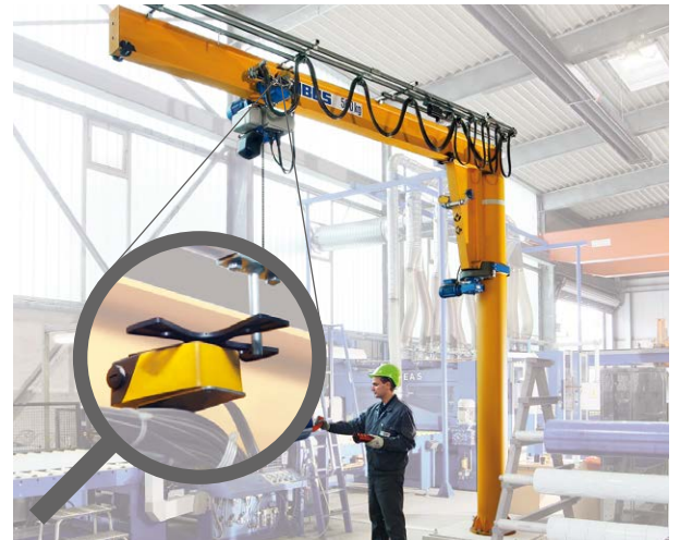
Limit switch for trolley travel (Fig. 8)
